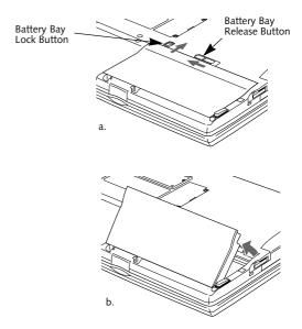
Figure 4-1 Replacing the Battery
